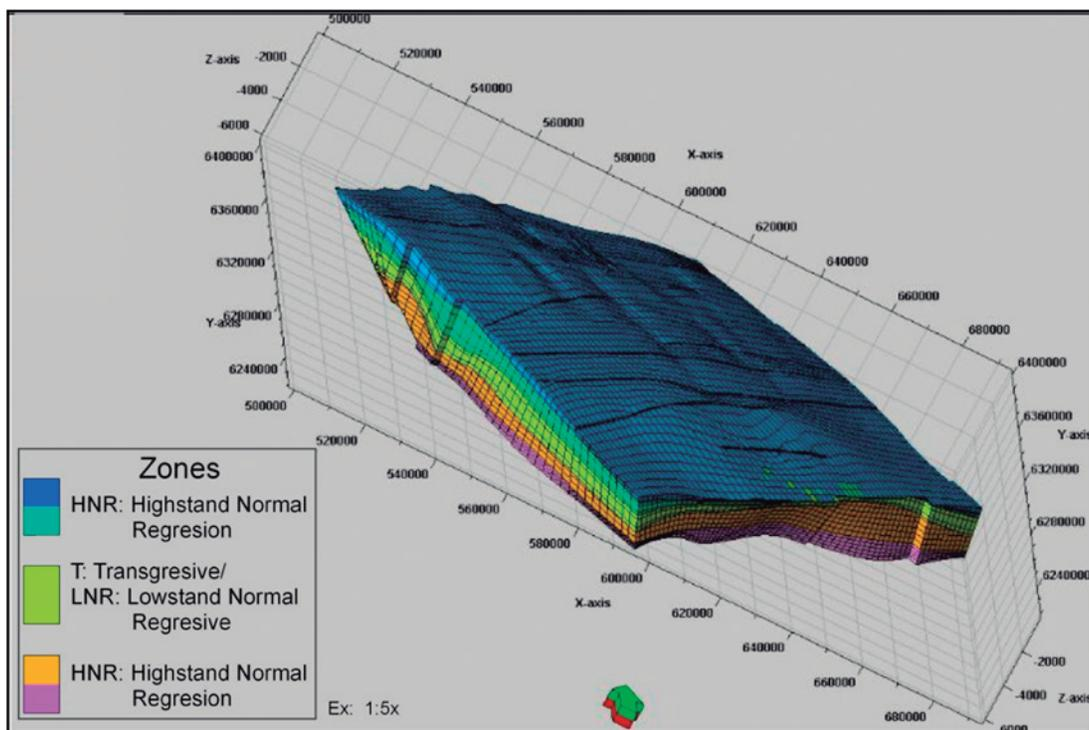
Figure 14. Three-dimensional computational model of the Rio Grande Cone, containing stratigraphic sequences, faults, channels and elements obtained from seismic interpretation.
