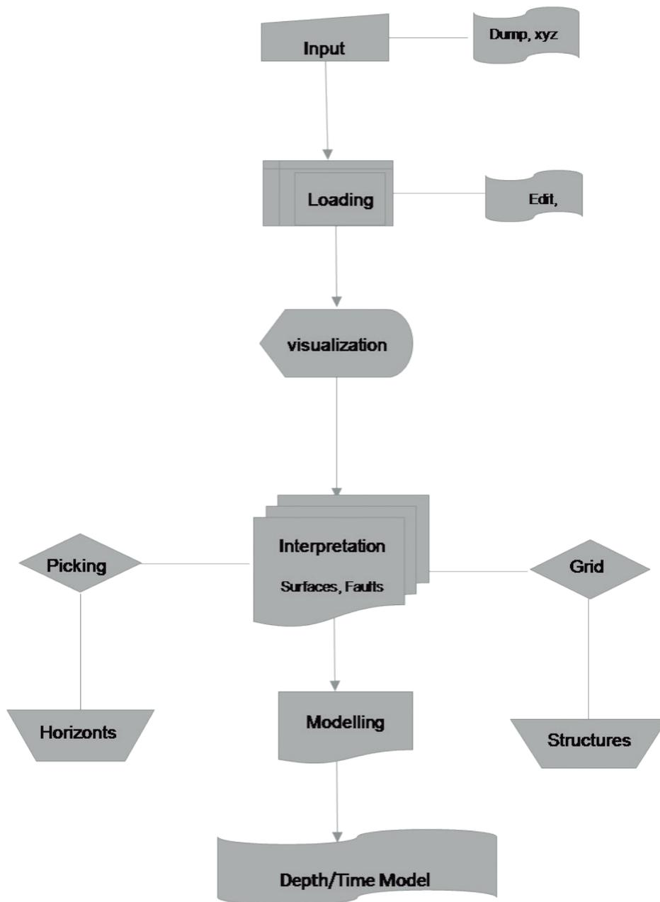
Figure 2. Chart diagram with different sequences used for seismic interpretation.
