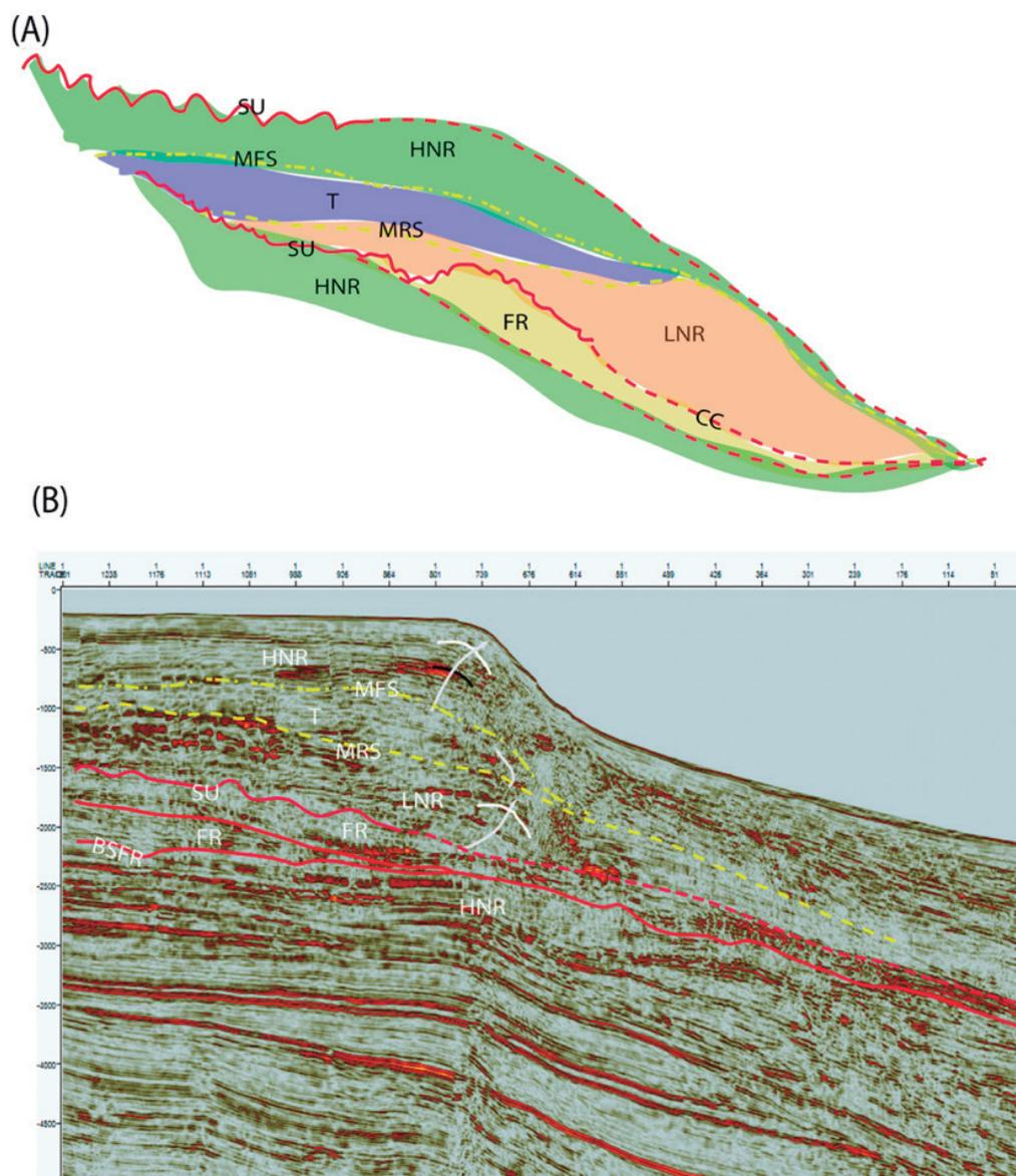
**Figure 5.** (A): Ideal schematic model representation of the sequence stratigraphy, with regressive and transgressive sequences (highstand, lowstand and transgressive). (B) Sequence stratigraphy interpretation in the dip regional seismic section located in the Rio Grande Cone, southern Brazil. The interpretation shows large-scale system tracts (based in Catuneanu *et al.*, 2008).
