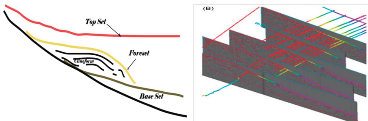
**Figure 9.** (A) Schematic representation of the termination and geometry of the clinoforms and sequences that determine the progradations found on the RGC, i.e., the topset, bottom and foreset; (B) dip seismic line interpretation (D1-lowest- to DVI) and interpretation of horizon and progradational sequences. The basal sequence is influenced by slumps, turbidities or gravitational flows characterizing the foreset sequence comprised of sediments, debris flows and mass transport complexes.
