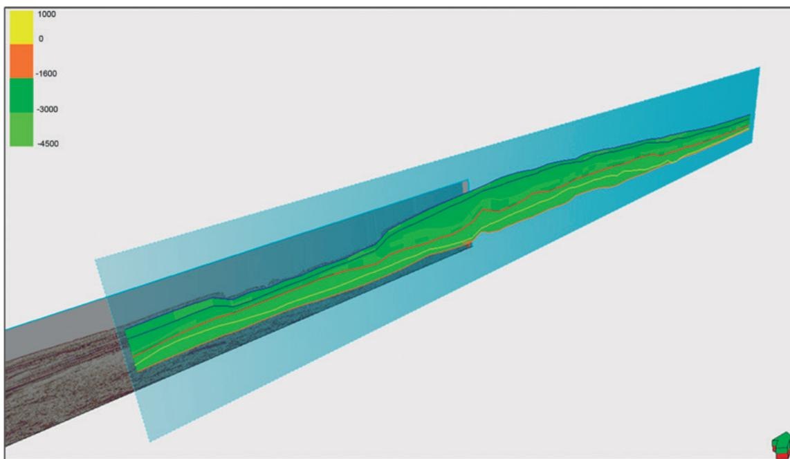
**Figure 11.** Regional dip lines with seismic interpretation describing the break shelf and clinoform and progradation sequences, showing lateral migration and pitch out toward the far offset. Surface lines correspond to possible lines for the velocity model and correlation.
