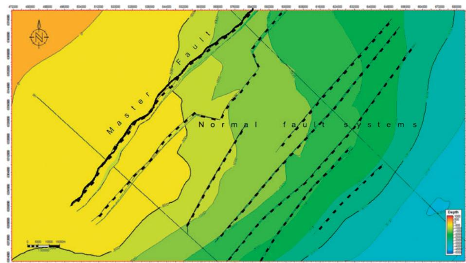
**Figure 6.** Plan view map with structural mapping of the principal normal faults and contours of the bottom surface. The principal or master fault corresponds to a listric fault (northwestern fault), while the other normal system faults are connected in depth to the master fault.
