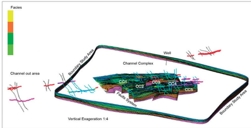
**Figure 12.** Seismic strike section and system channel complex identification. Channel position after geobody modeling.
