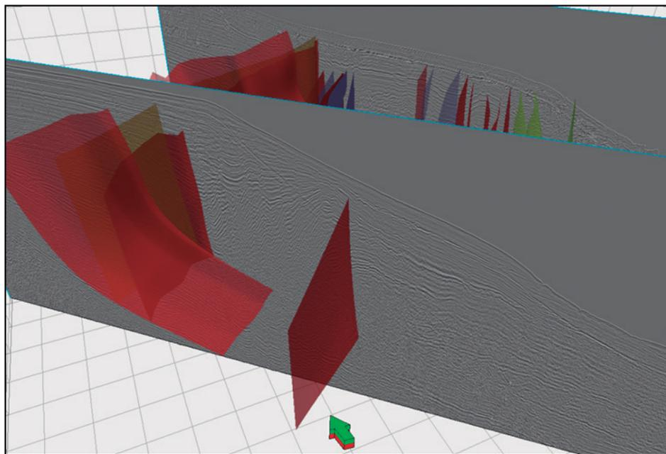
**Figure 7.** Three-dimensional structural model with features identified in the Rio Grande Cone using seismic sections. The section includes regional normal faults, strike slip faults and vertical faults; the model illustrates fault system planes crossing all sequences of the RGC sedimentary package.
