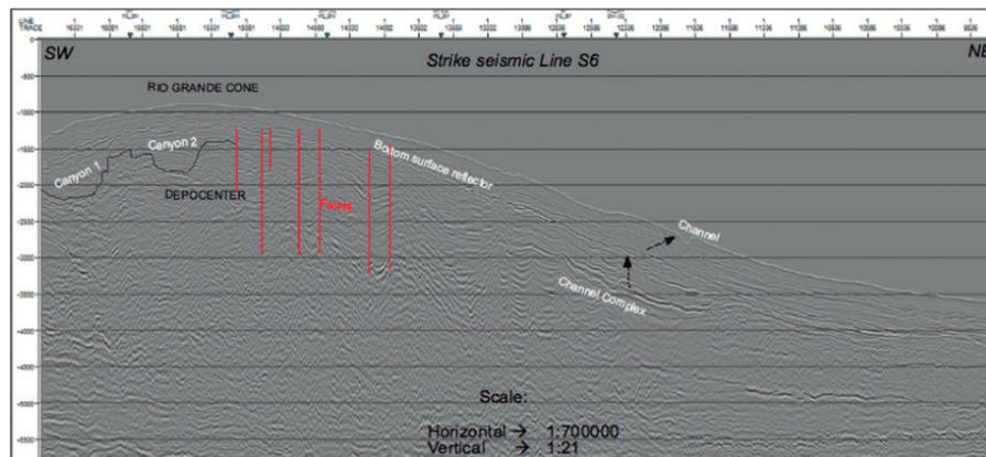
Figure 4. Strike seismic section (S6) line with sequential stratigraphic interpretation from the Neogene interval in the Rio Grande Cone, with the depocenter and migration of complex channels influenced by sediment supply, eustasy and accommodation.
