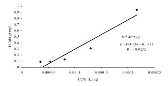
Figure 6. Obtained of Kd for the silica sand. Figura 6.  $K_d$  obtenido para la arena sílice.
