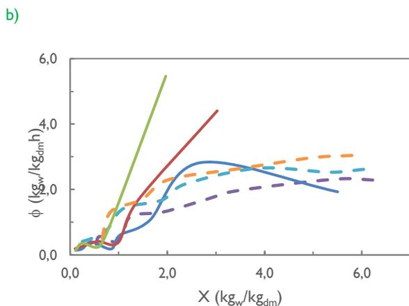
**Figure 1.** Drying curves of *yacón* for the two studied methods at different temperatures: a) moisture vs. time, b) drying rate curve. CD: convective drying, ID: far-infrared drying.
