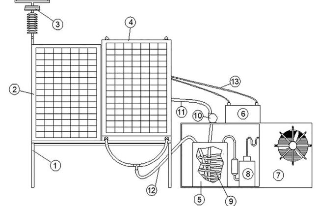
**Figure 3.** Experimental setup and its parts: 1) scaffold, 2) PV module, 3) weather station, 4) PV-T module, 5) water tank, 6) battery, 7) fan, 8) compressor, 9) serpentine, 10) pump, 11 and 12) PE pipes
