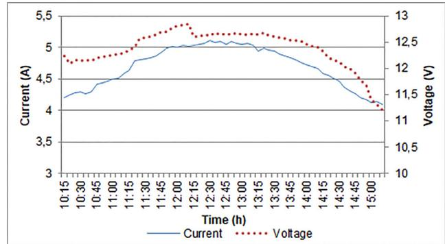
**Figure 6.** PV-T module with cooling, current-voltage graph (24 June 2019)
