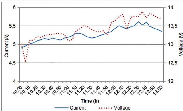
Figure 9. PV-T module without cooling, current-voltage graph (30 June 2019)
