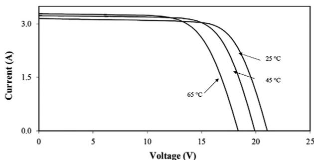
**Figure 1.** Influence of temperature on a PV module I-V curve
