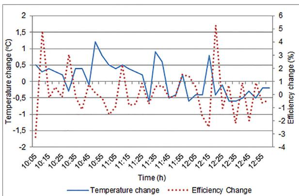
Figure 11. PV-T module without cooling, temperature-efficiency graph (30 June 2019)
