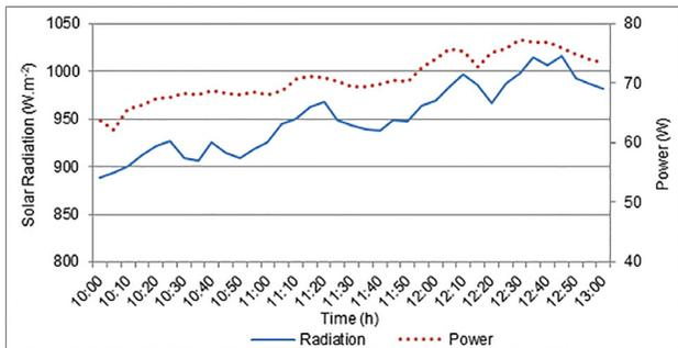
Figure 10. PV-T module without cooling, solar radiation-module power generation graph (30 June 2019)
