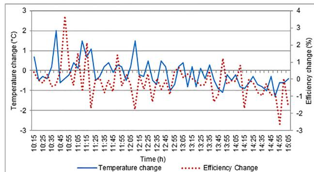
**Figure 8.** PV-T module with cooling, temperature-efficiency graph (24 June 2019)
