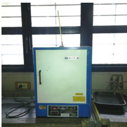
Figure 2. Gravity convection oven used to perform the accelerated thermal aging test
