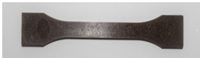
Figure 1. Type 1B 527 ISO standardized specimen (ASTM D638-14) made of PP/20F biocomposite, from which the samples for the study were extracted
