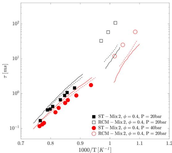
**Figure 4.** Ignition delay for natural gas mixture. Experimental data (symbols). Numerical data (lines) using the LLNL (straight) and NUIG mechanisms (dashed).
