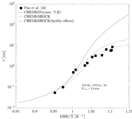
**Figure 9.** Ignition delay predictions for  $H_2$ , as improved using CHEMKSHOCK
