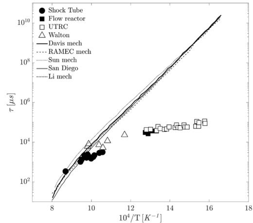
**Figure 5.** Experimental and numerical ignition delay values for  $\text{H}_2$
