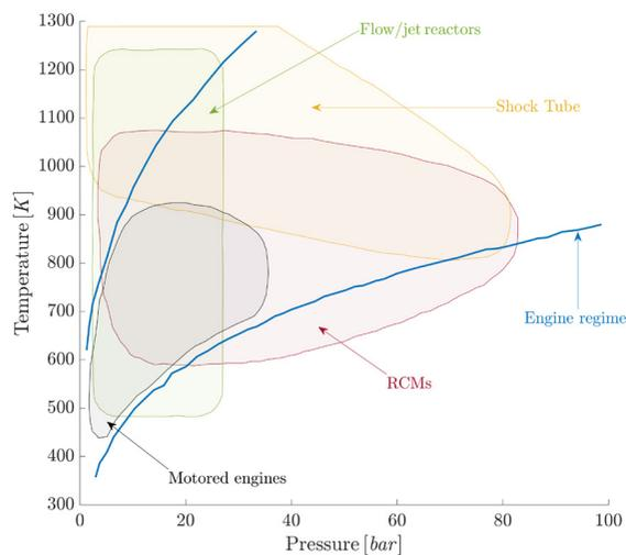
**Figure 1.** Operating ranges of the devices used for  $\tau$  measurements
