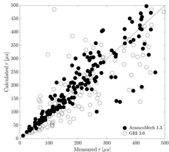
**Figure 2.** Ignition delay comparison for  $\text{CH}_4/\text{C}_2\text{H}_6/\text{C}_3\text{H}_8/\text{H}_2$  mixtures
