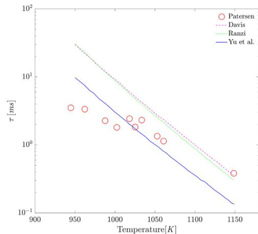
**Figure 6.** Ignition delay for a syngas mixture
