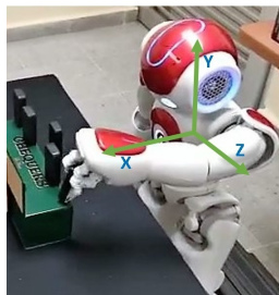
Figure 13. Reference coordinate system on the NAO robot's arm
