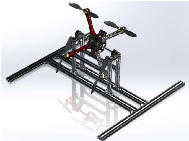
Figure 4. CAD assembly of a one-degree-of-freedom test bench Source: Authors
