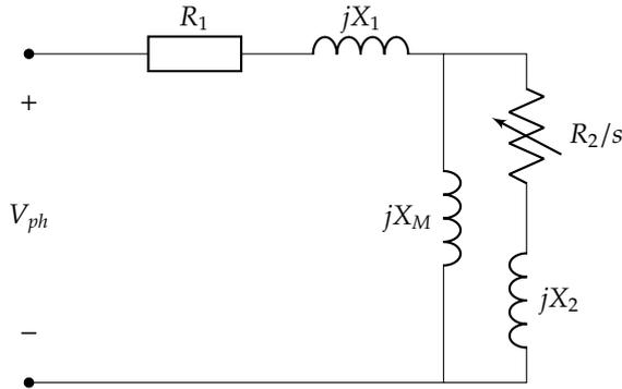
Figure 1. Single-phase equivalent of the induction motor
