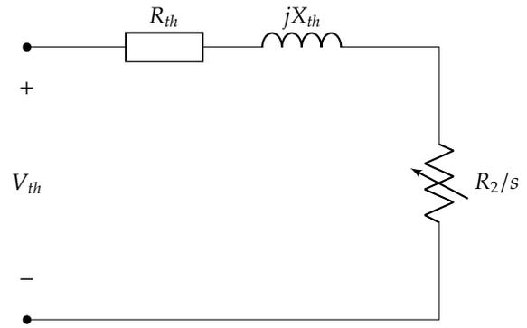
Figure 2. Thevenin equivalent of the single-phase circuit of the induction motor
