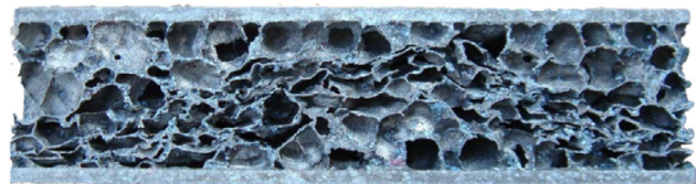
Figure 4. Surface obtained via the wire erosion cutting of sandwich plates
