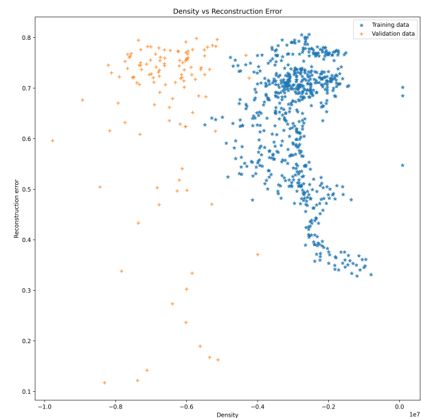
Figure 7. Scatter plot obtained from the KDE and RE values of the VGG16 autoencoder. The orange crosses are the anomalous points (defective limes), while the blue stars correspond to the healthy fruit. Source: Authors
