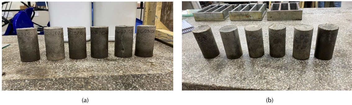
Figure S5 – (a) Test specimens with GO addition, after demolding; and (b) Test specimens without GO addition, after demolding.
