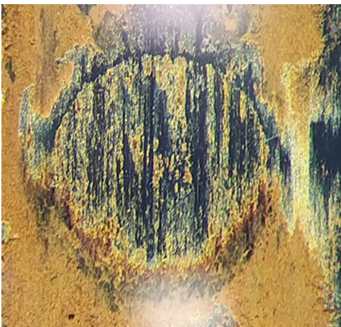
Figure 15. Track dry wear test with stereoscope Source: Authors
