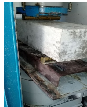
Figure 4. Beam flexure test.
