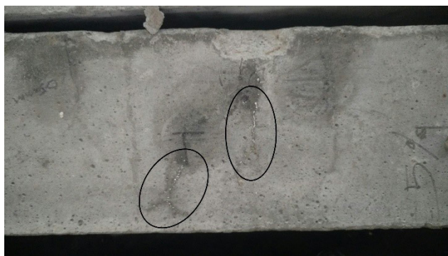
Figure 7. Healed bacteria-enriched SFRSCC
