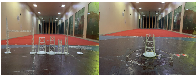
Figure 5. Experimental models constructed by 3D printing: (a) Experimental models; (b) Model A in testing Source: Authors
