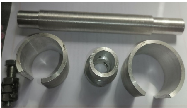
Figure 6. The fabricated prosthesis limb parts were processed in the turning machine Source: Authors
