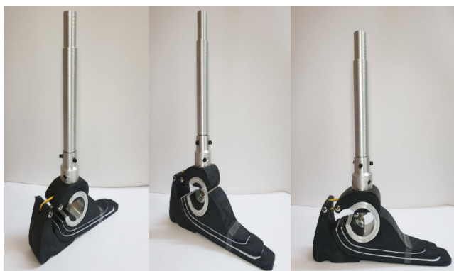
Figure 9. Final assembly of the smart prosthetic leg prototype Source: Authors
