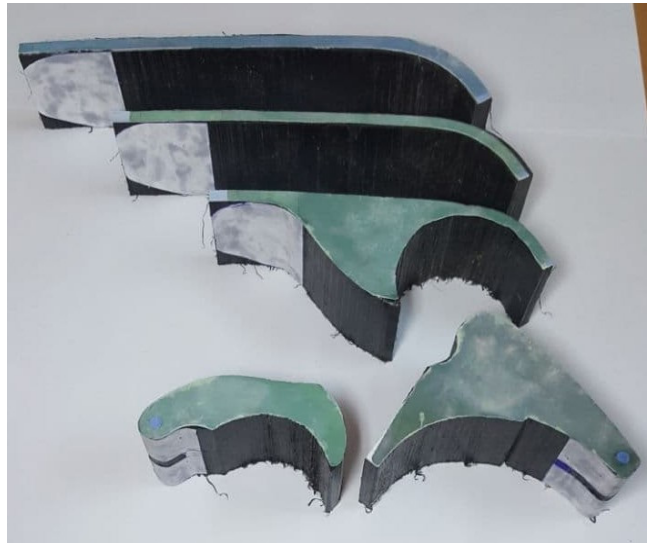
Figure 7. Cutting the parts of the artificial foot using a band saw machine Source: Authors
