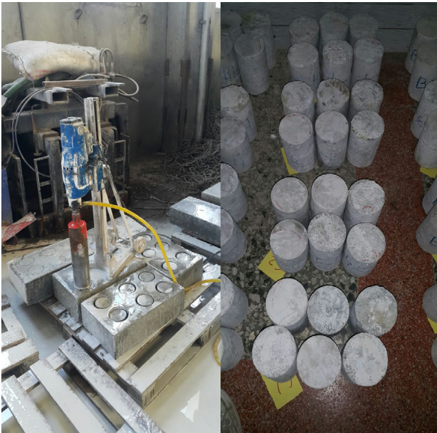
Figure 4. Data preparation: a) coring process; b) core samples whose surface images were taken Source: Authors
