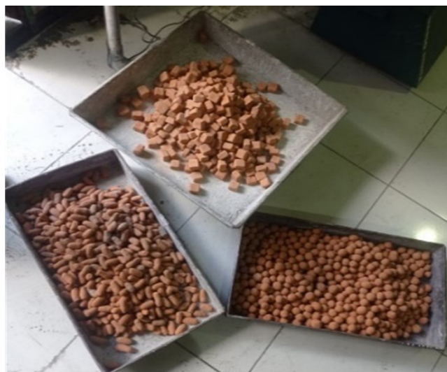
Figure 2. Shape of the coarse aggregates
