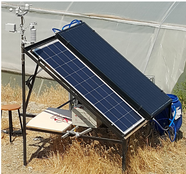
Figure 3. Experimental setup and its parts: 1) scaffold, 2) PV module, 3) weather station, 4) PV-T module, 5) water tank, 6) battery, 7) fan, 8) compressor, 9) serpentine, 10) pump, 11 and 12) PE pipes Source: Authors
