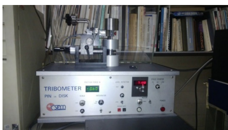
Figure 3. Tribometer used for the study of sliding wear
