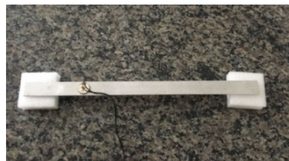
Figure 1. Aluminum beam and PZT patch used in the experiments Source: Authors
