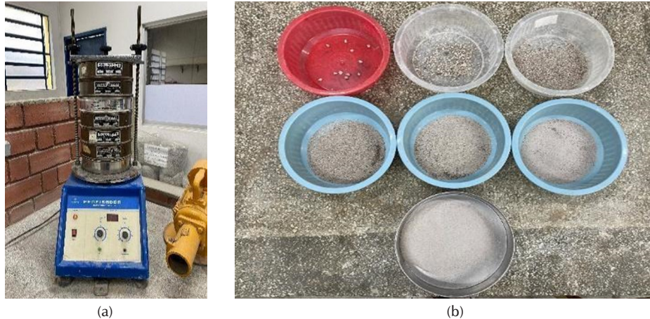
Figure S1 - (a) Mechanical sieve and (b) - Granulometry test Source: Authors
