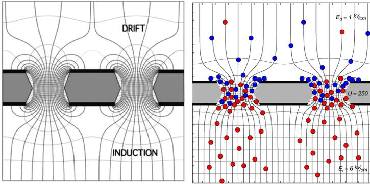
FIGURE 2. The electric field in the region of the holes of a GEM electrode [1].
