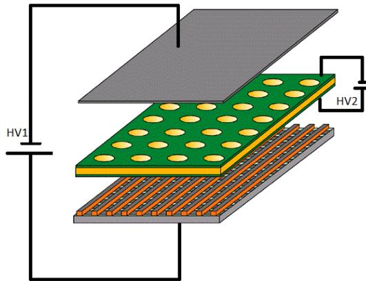
FIGURE 1. Schematic view of a single-GEM detector [1].
