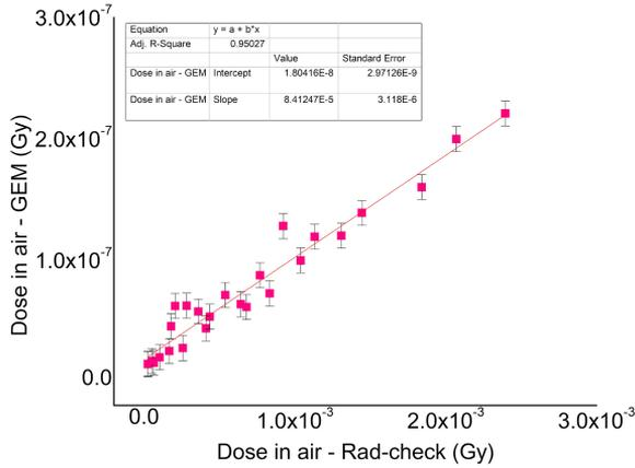
FIGURE 6. Dose in air as measured with the triple-GEM detector compared to reference dose measured with the Rad-check ionization chamber. The linear fit provides the calibration function that allows to correct dose measurement done with the triple-GEM detector with the calibration coefficient  $1.13 \times 10^4$ . The horizontal error bars are too small to be visible in the graph because of the high precision of the Rad-check detector.
