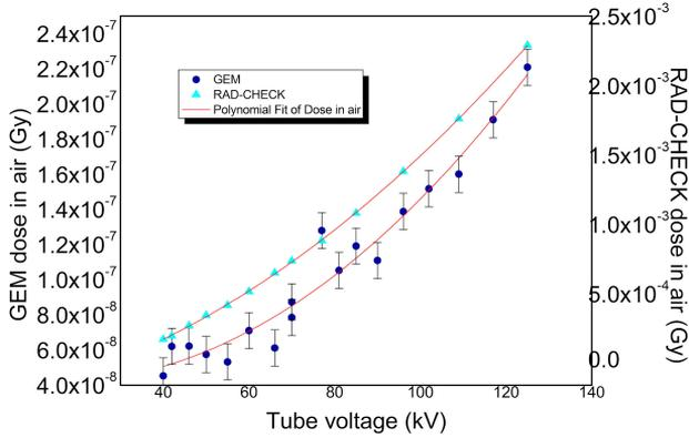
FIGURE 4. Dose in air vs tube voltage measured with the triple-GEM detector compared to the reference dosimeter. Measurements were made at a distance (SOD) of 88 cm, tube current of 16 mAs, and detector HV of -4200 V. The relationship is quadratic despite high dispersion at low voltages.
