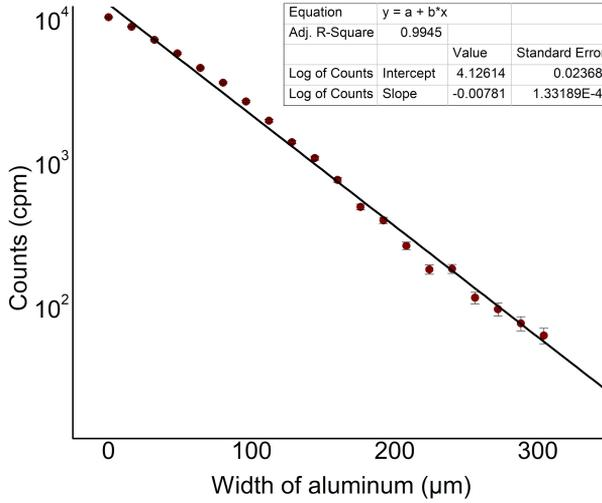
FIGURE 3. Counts vs thickness of aluminum filters ( $x$ ), taken on the triple-GEM detector. It shows the linearity of the detector's response as a function of the intensity of the photon beam.
