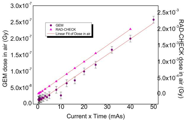
FIGURE 5. Dose in air vs tube current measured with the triple-GEM detector and the reference detector. Measurements were made at an SOD of 88 cm, peak tube voltage of 73 kVp, and detector HV of -4200 V. Both sets of data are well fitted to a linear function. The Rad-check data has an  $R^2$  of 0.99992, while the GEM's is 0.98588.
