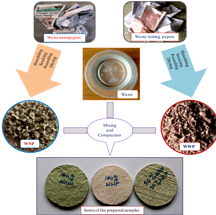
FIGURE 1. Summary of the sample's fabrication processes
