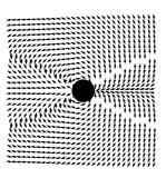
FIGURE 3. Force that does terrestrial magnetic field upon solar wind in the plane y = 0; the solar wind comes from left to right. We have taken k = 0,005 $u^{-1}$  and m = 1.
