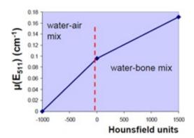
Figure 2. Relationship between PET attenuation coefficient values and CT Hounsfield units.
