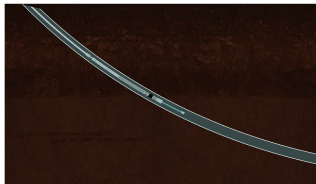
Figure 7. Lowering the fracturing device through the tubing column.
