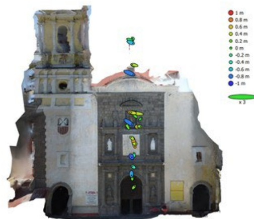
Fig. 3. Camera locations and error estimates. Z error is represented by ellipse color. X,Y errors are represented by ellipse shape. Estimated camera locations are marked with a black dot.
