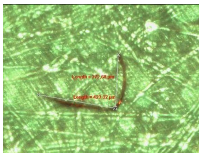
Figure 2. Dimension of a microplastic fragment using an inverted microscope (10× magnification). The fragment dimensions were obtained with NIS image analysis software. The sample was analyzed under fluorescence illumination.
