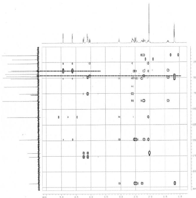
Figure 2. HMBC (long-range <sup>13</sup>C-<sup>1</sup>H correlations) spectrum of compound **2**.
