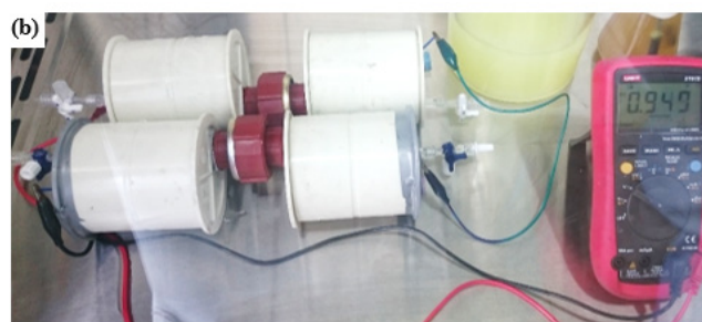
Figure 2. MFC-MEM. (a) Scheme used in the experiment. O.M: organic matter. (b) Real mfc-mem used.
