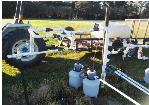
Figure 4. Inoculated pond water tank and the filtration system, integrating sand and zeolite.
