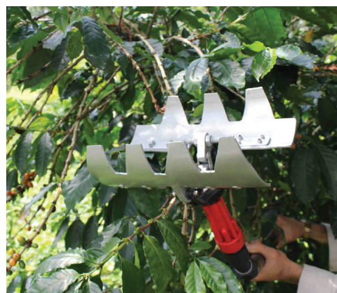
Figure 2. The Italian-made MAIBO beater (A) and the beater designed by Cenicafé-CENICAFE-I (B).
