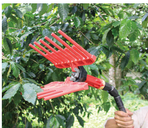
Figure 2. The Italian-made MAIBO beater (A) and the beater designed by Cenicafé-CENICAFE-I (B).
